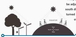
The panel should be adjusted in the south direction and turned at an angle of 40°.
